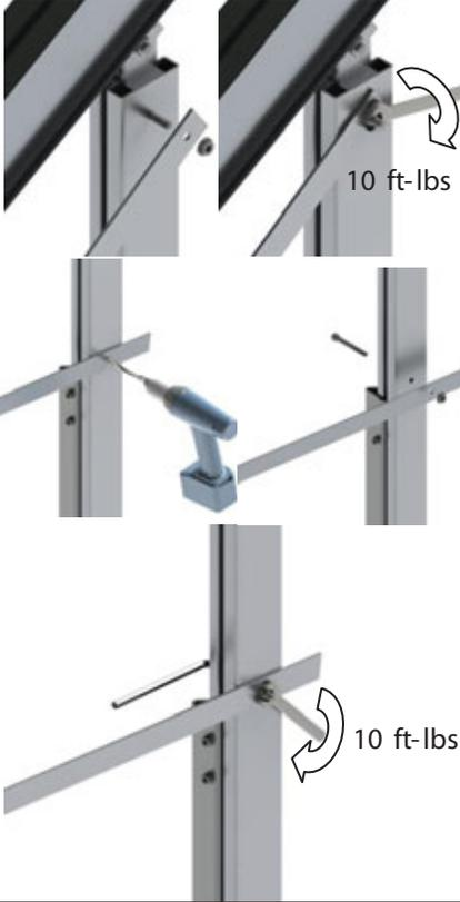
Note : The M10 hardware and Diagonal Strap can be installed on either side of the Vertical Post.
