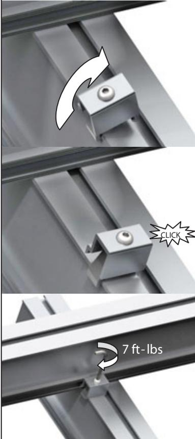
Attach the 120/90 Top Rail **[E]** to the bottom rail using the Cross Adapter **[G]**. This requires at least 2 cross adapters per connection (may require 4, depending on site conditions). Click the Cross Adapter onto the rail, slide up to the top rail and fasten the bolt by turning clockwise.
